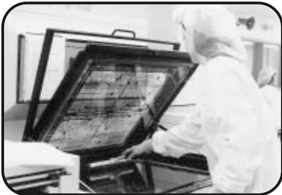
All photographic printing areas at ACI are inside cleanrooms to control errors due to dust and dirt.
