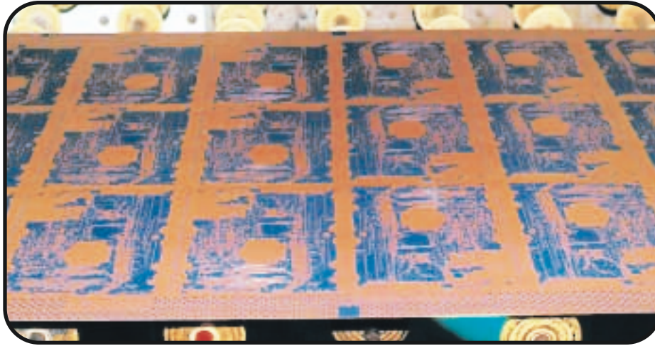
The resist on inner layers protects the copper under it from the etching process.
