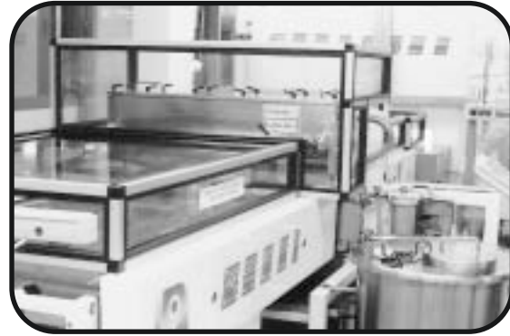
Resist is applied to inner layers as they pass through a sheet of liquid resist. The coating is then cured in an oven.
