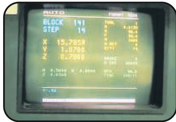
The precise location of each hole or rout path is specified by programs generated in Process Engineering. They are then downloaded into a computer-controlled driller or router.
