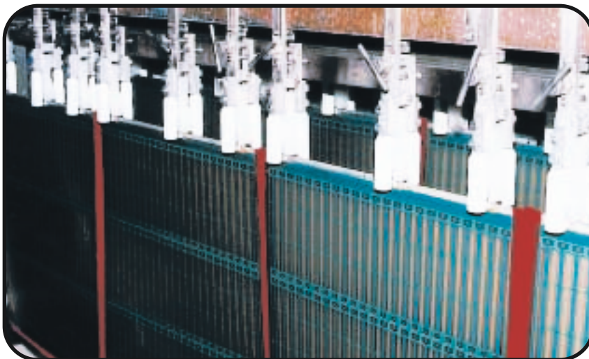
Electroplating requires an electrical connection to the panel.
