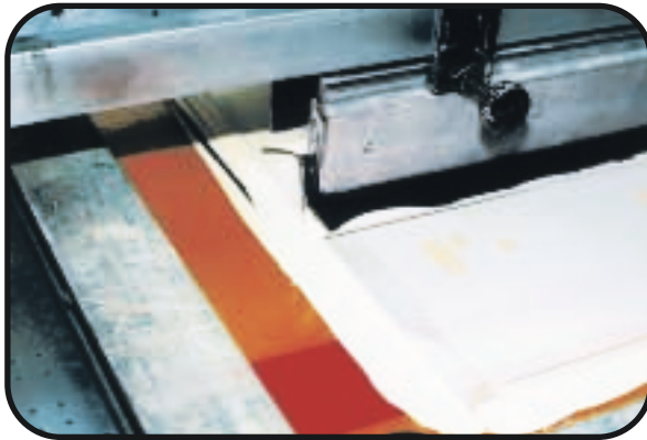
As the squeegee passes over the screen, ink is forced through the open holes and is deposited on the panels.
