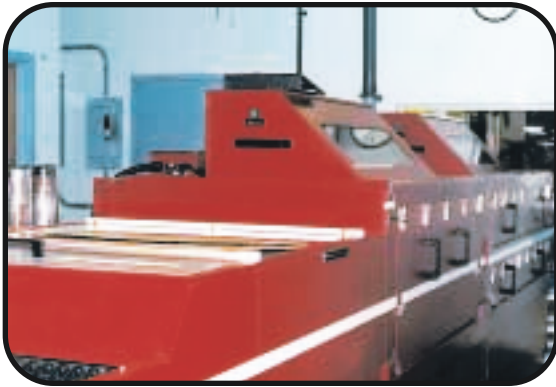
A developer completes the printing process by removing the unexposed resist.
