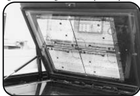
Phototools are cleaned and held against a glass frame by vacuum. Panels or layers are placed between two phototools and exposed to ultraviolet light.
