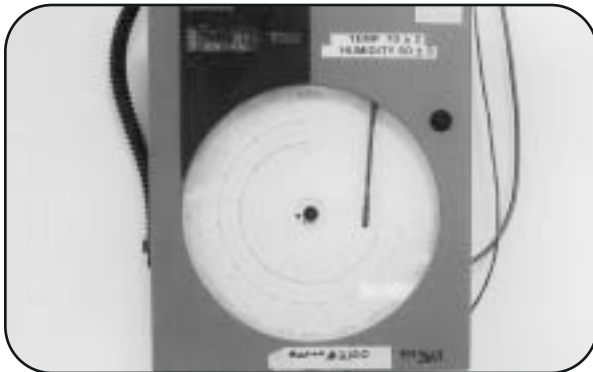
Temperature and humidity are tightly controlled and monitored to minimize misregistration due to changes in the size of phototools.
